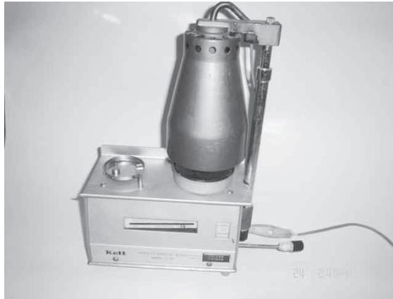
Gambar 23 *Infrared Moisture Meter* model F-IA Kett
