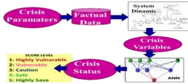
Fig.3 The computational intelligent engine of the EWS sub-system (Seminar et al. 2010).
