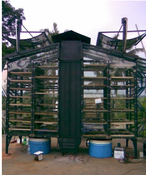
Figure 1. The green house effect solar dryer
