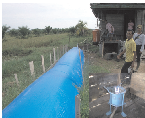
Figure 3. Simple biodigester made from plastic
