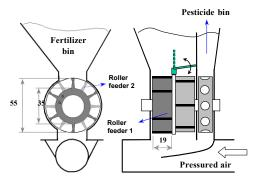
Figure 3. Schematic of metering device
