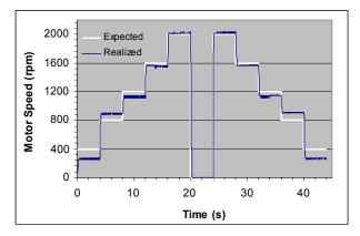
Figure 9. Step response of motor without control
