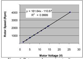
Figure 6. Rotor speed versus input voltage
