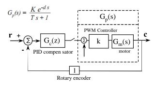
Figure 6. Schematic diagram of digital control
