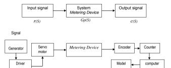
Figure 5. Schematic of system identification
