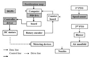
Figure 2. System control of variable metering.
