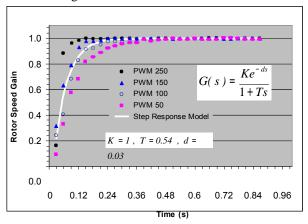
Figure 8. Step response model of system
