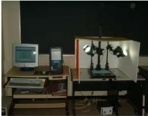
Figure 1 The light-controllable image capturing chamber
