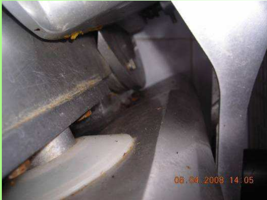
Dirty equipment, poor cleaning method
