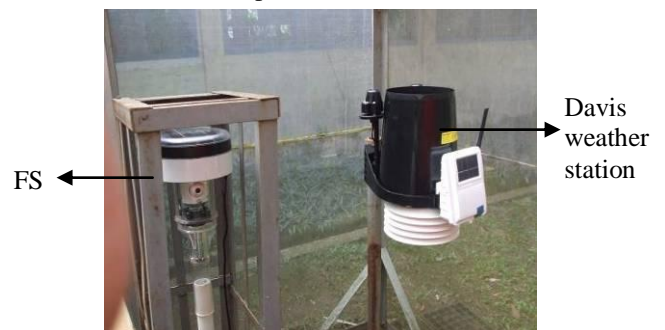
Gambar 2. Kalibrasi Field Server (FS)
