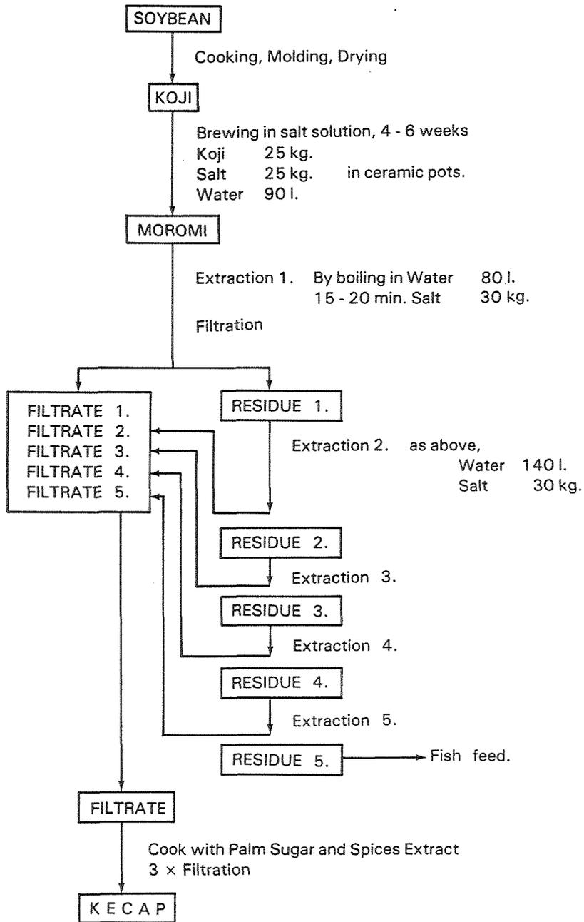
Fig. 3. General Flow Chart of Kecap Manufacturing Process.
