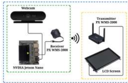
Gambar 3 Sistem Pendeteksi Tanah Berbasis Artificial Intelligence
