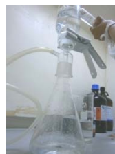
Figure 17 Vacuum pump for mobile phase preparation
