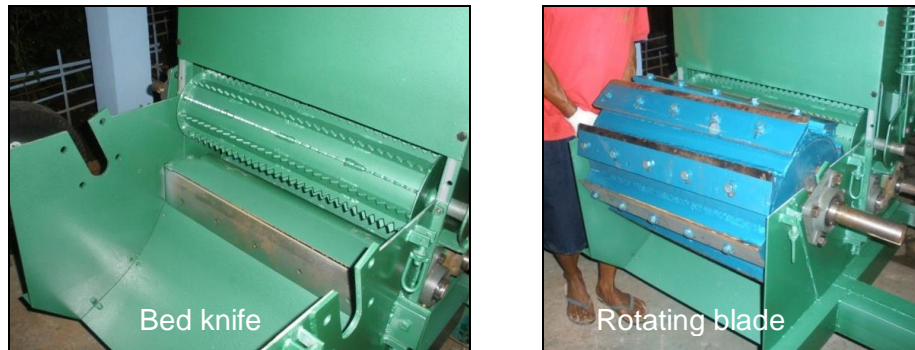
Figure 9. The prototype of the leaf trash chopper section.
