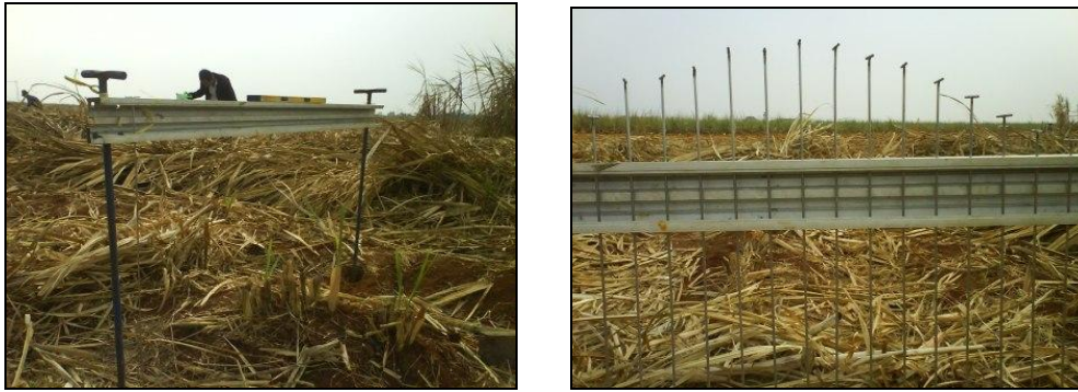
Figure 2. Measurement of leaf trash conditions and ridge profiles using a reliefmeter.
