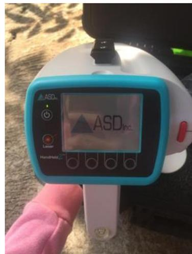
Gambar 3 Alat *HandHeld 2 Spectroradiometer*
