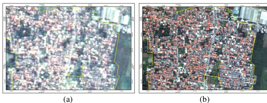
Figure 4. Difference of delineation of land and building area from different image resolution: a. ALOS-AVNIR, and b. IKONOS
