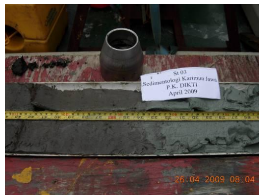
Figure 4. Sediment from gravity core sample
