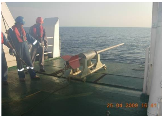
Figure 3. Gravity core sample tool
