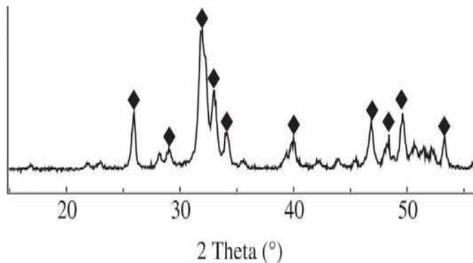
Figure 2 XRD pattern of HA from wet precipitation method (◆ HA) (Santos *et al* 2004).
