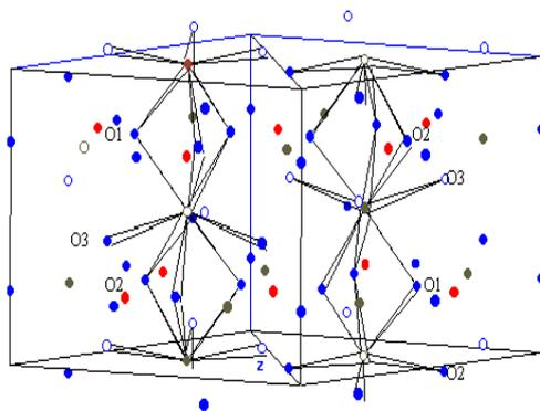
Figure 1 The crystal structure of hydroxyapatite (Shi *et al* 2004).
