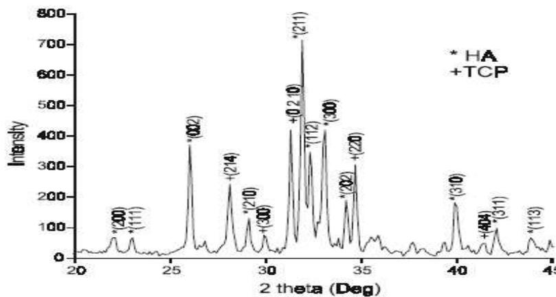
Figure 3 BCP X-Ray Diffraction Pattern from 900°C sintering (Kumar *et al* 2005).
