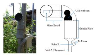
Figure 5. The chassis for USB webcam
