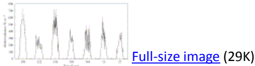
Fig. 3. Model calibration for 7 non-successive days. Time courses of the global radiation transmission through the greenhouse: —, measured; - - - - -, calculated.
