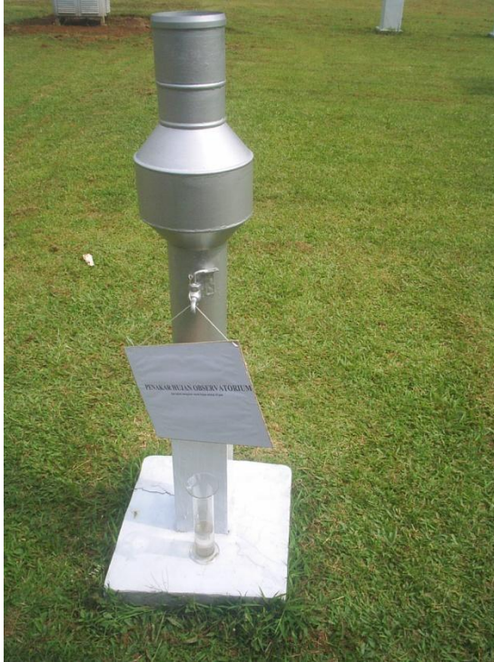
Gambar 1. Alat Standar Penakar Hujan Observatorium
