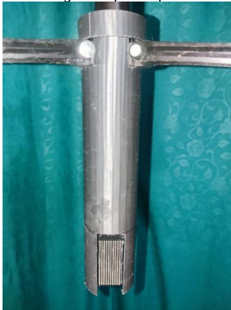
Gambar 26 Casing Kaki Sistem Berisi Water Level Sensor K0135
