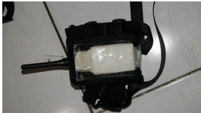
Gambar 3.12. Prototype GPS Tracker Final & Harness.
