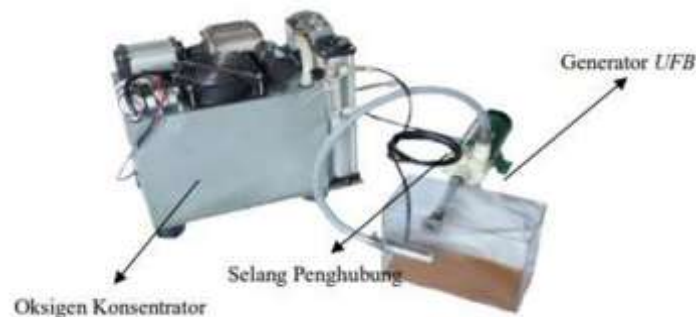
Figure 1. Oxygen concentrator and ultrafine bubble generator used for biodiesel treatment (reproduced from Farafisha, 2023).
