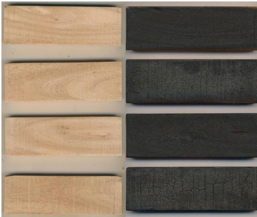
Figure 7 Appearance of mindi wood surface before and after burning.
