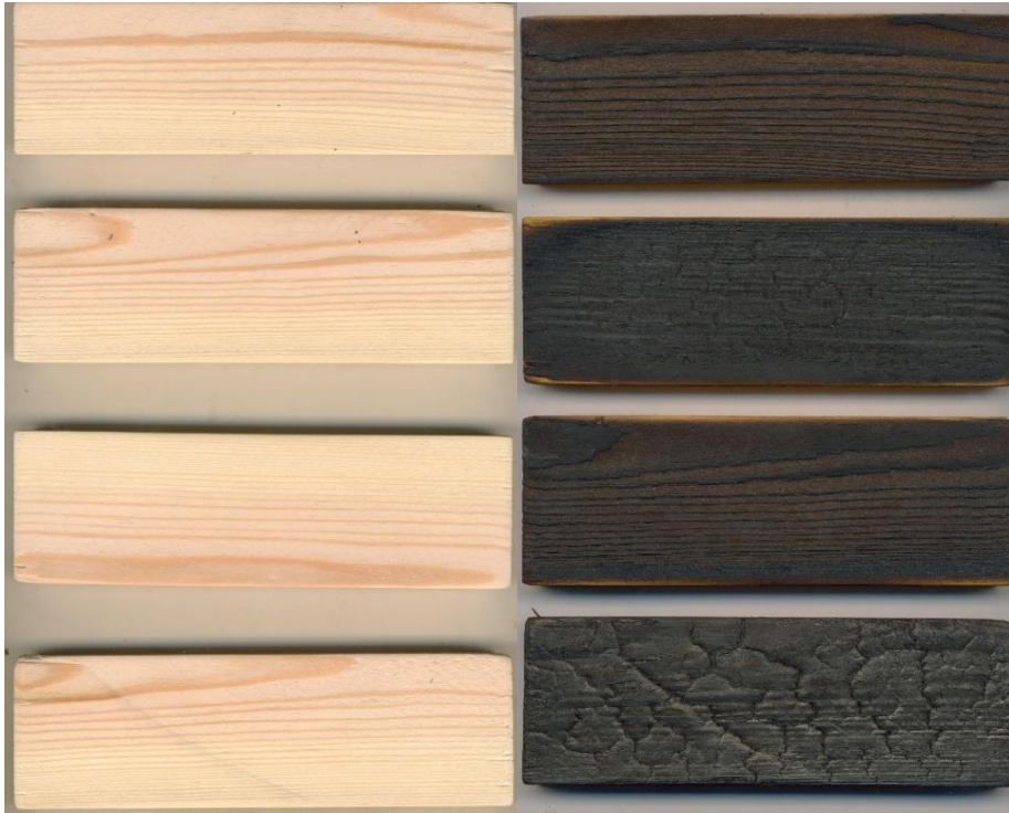
Figure 8 Appearance of pine wood surface before and after burning.
