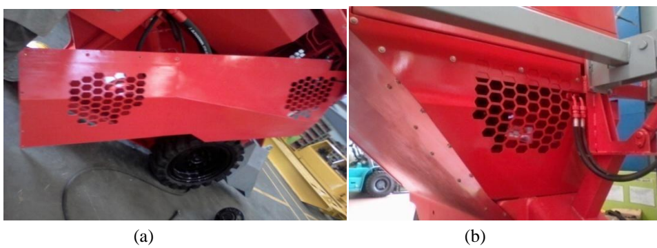
Gambar 26. Cover frame : (a) cover bagian samping frame , (b) cover bagian depan frame
