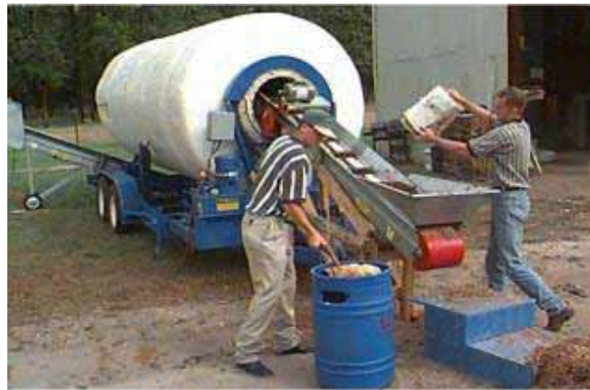
Gambar 7. Rotary drum composters (Isro'i 2004)
