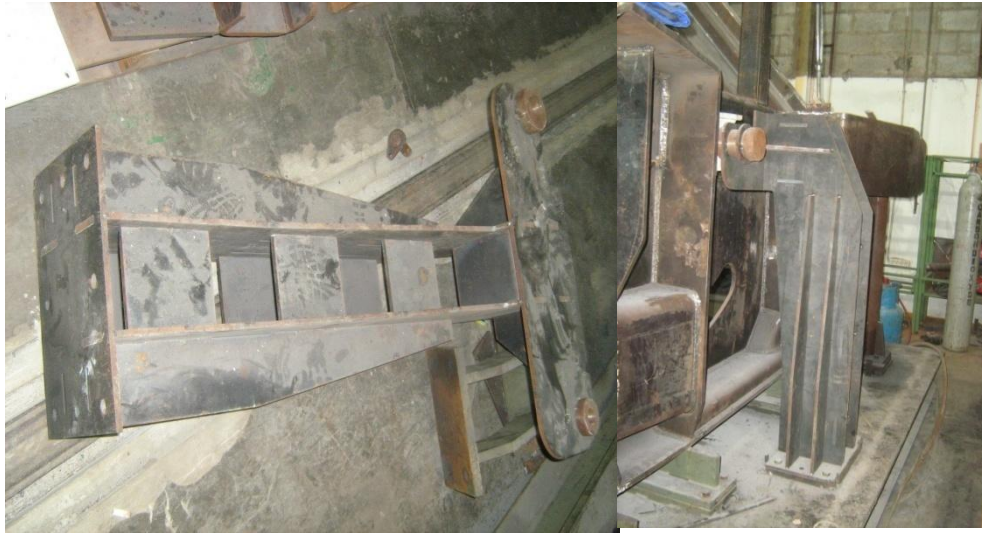
(a) (b) Gambar 58. Jig komponen drum blade : (a) jig saat dilepas, (b) jig saat terpasang
