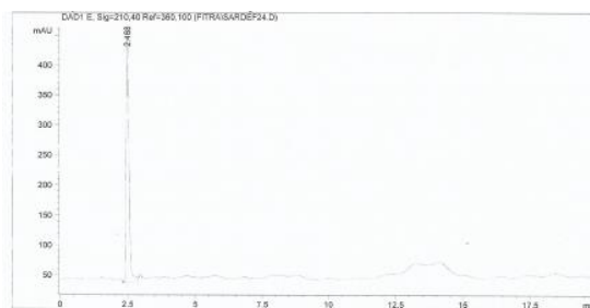
Figure 3. Chromatogram alkaloid compounds HPLC standard (atropin) with phase motion 10% and 90% acetonitrile \text{KH}_2\text{PO}_4 0.01 M in water (pH 3), isokratis, elusi column RP-18e, injection volume, flow rate 20 \mu\text{L} of 1.0 mL/min, UV detector at a wavelength of 280 nm.
