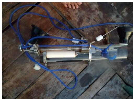
Gambar persiapan pengambilan sampel air    Gambar *Vann dorn water sampler*
