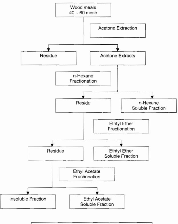
Figure 1: Schematic fractionation of acetone extracts
