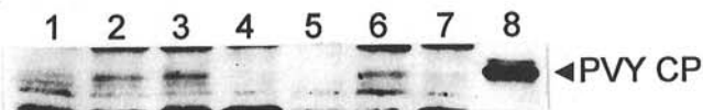
Fig. 2. Western blot of total protein from green leaf tissue obtained from independent transgenic R 0 plants carrying the potato virus Y (PVY) Chilean isolate coat protein (CP) gene. The blot was probed with PVY antiserum. Lanes 1 and 4, nontransformed KY14; lanes 2 and 3, KY14-5C-R; lane 5, NC3433-33-13C-2-S1; lane 6, NC 3433-33-1TH-S1; lane 7, nontransformed NC3433-33; and lane 8, 0.01 µg of PVY CP.
