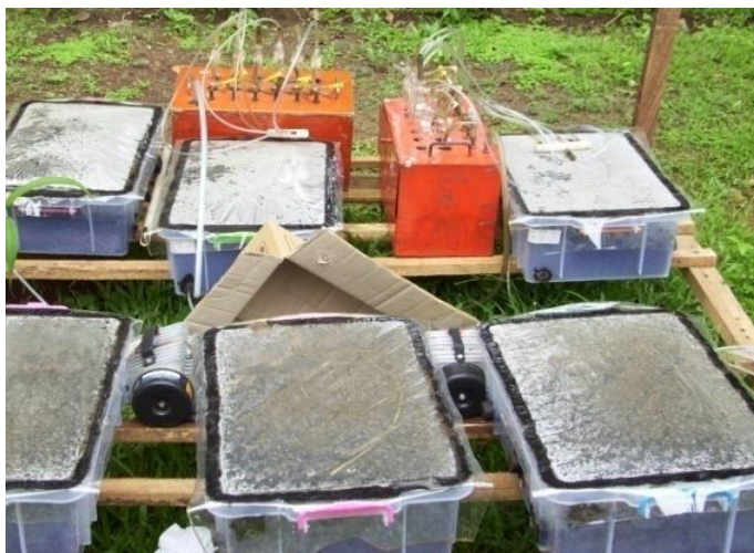
Figure 1. CO 2 and NH 3 sampling during the landfarming bioremediation process.
