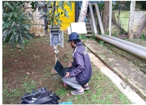
Panel Water Level Logger WL16U-030-050 di PT Aqua Golden Mississippi
