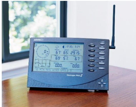
Receiver AWS tipe Davis Vantage Pro 2
