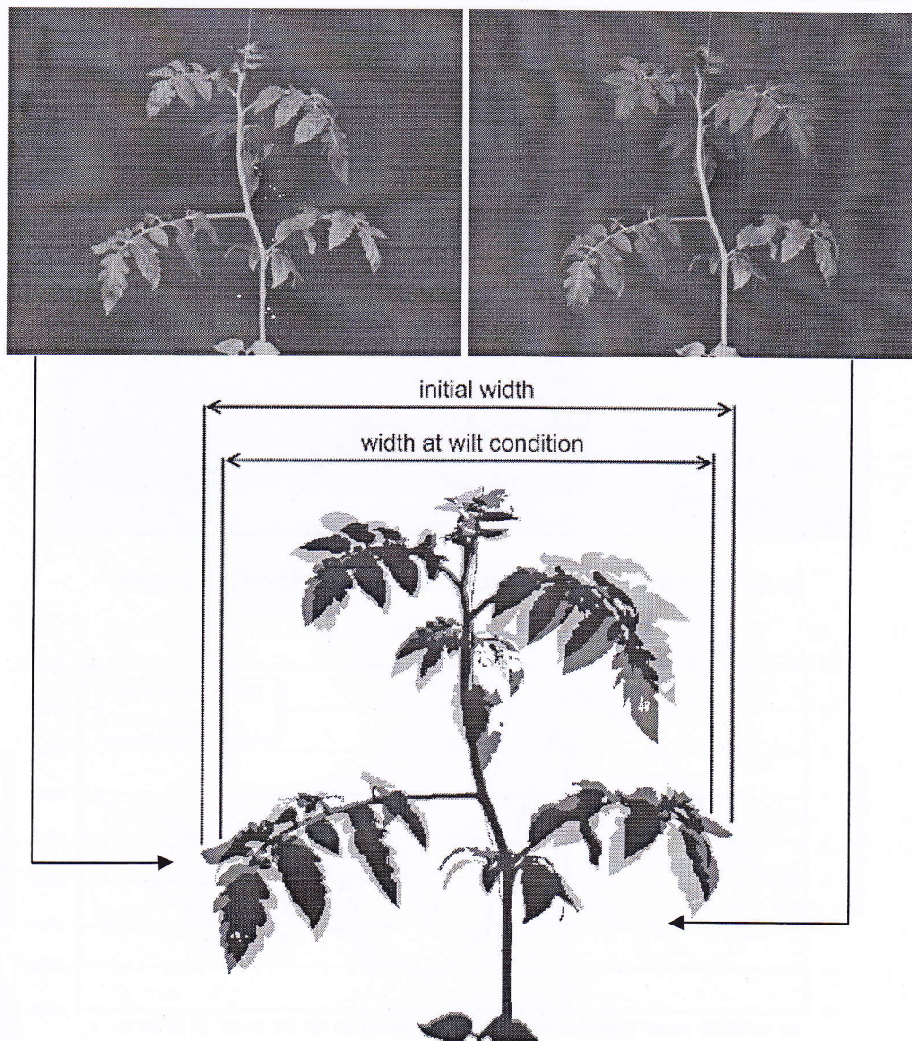
Figure 4. Measurement of comparison of width of the plant in image. (Dark gray is original condition, light gray is wilt condition, and black is overlapped part of the two images)
