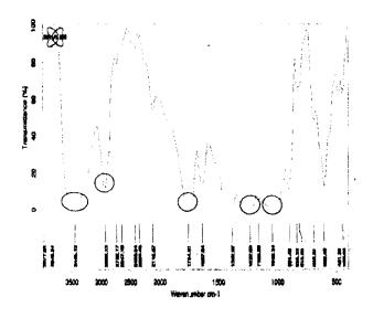
Figure 5 FTIR Spectra of CA Membranes.
