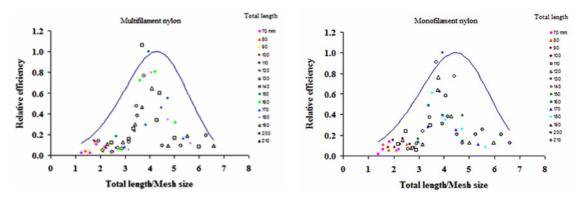
Figure 8. The Master Curves of Mesh Selectivity of the Trammel Nets (Multifilament and Monofilament Nylon Inner Nets) in Term of Length Ratio to Mesh Size (I/m ratio) for Amoy Croaker
