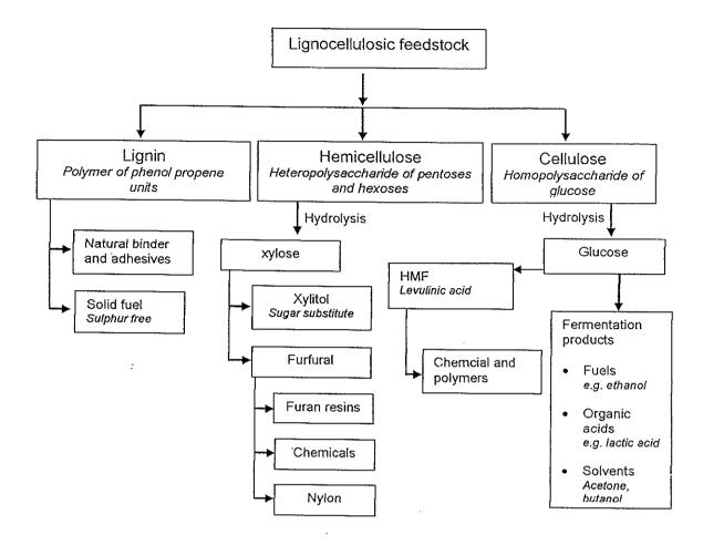
Figure 1. Lignocellulosic feedstock bio-refinery (adapted from Kamm *et al.*, 2004)
