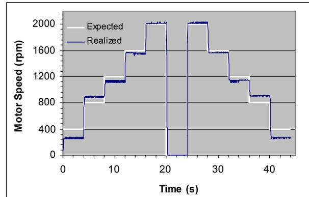
Figure 9. Step response of motor without control
