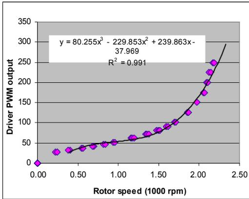
Figure 7. PWM output of motor driver versus rotor speed
