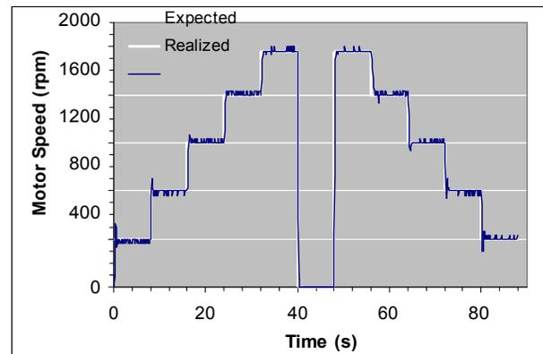
Figure 10. Stair step response of motor with PID control
