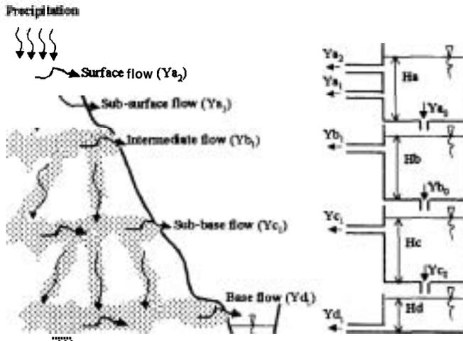
Gambar 1. Skema representasi Tank Model
